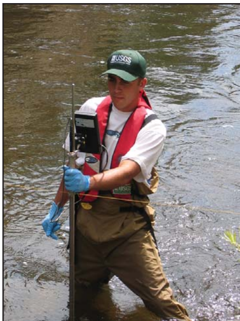
Jason Gurdak, USGS Hydrologist, uses a current meter to measure stream discharge in the Big Thompson River.
